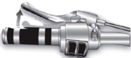
**Friction zone** – the point on the clutch where the engine’s power begins to transmit to the rear wheel.
