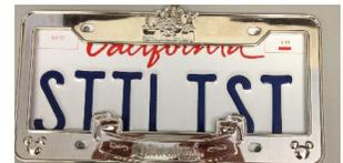
When characters are located too close to the plate's edge, license plate frames can easily prevent the plate number from being read by an LPR.
