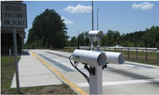
LPR camera in use at a roadside truck scale.
