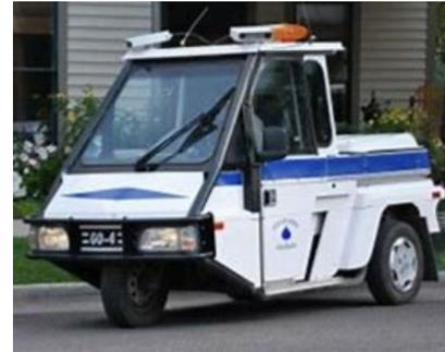
Mobile LPR camera mounted on parking enforcement vehicle.
