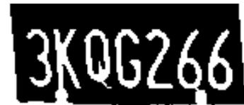
The segmented or pre-processed license plate image is then passed off to OCR software, where the images are converted to individual alphanumeric characters.
