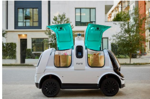
The Nuro R2 zero-occupant autonomous delivery vehicle, designed to carry goods on public roads. It fits the federal low-speed vehicle classification and has received a US Department of Transportation and the National Highway Traffic Safety Administration regulatory exemption from some Federal Motor Vehicle Safety Standards regulations for usage on public roads.
