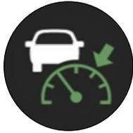
**Description:** Can increase or decrease the vehicle's speed to maintain a following distance set by the driver. Advanced versions can even slow and stop the vehicle in traffic jams and then accelerate automatically.
