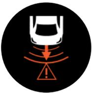
**Description:** Uses rear sensors to scan for objects behind the vehicle and alerts the driver if an object is detected.
