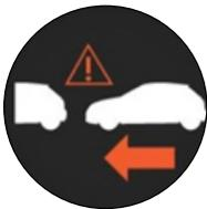
**Description:** Can sense slow or stopped traffic or an object ahead and urgently applies the brakes if the driver fails to respond.
