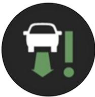
**Description:** This feature monitors traffic when the driver turns left across traffic at low speeds (such as at a traffic light). It activates warning sounds and dash lights and automatically applies the brake if a driver is turning left into the path of another vehicle.
