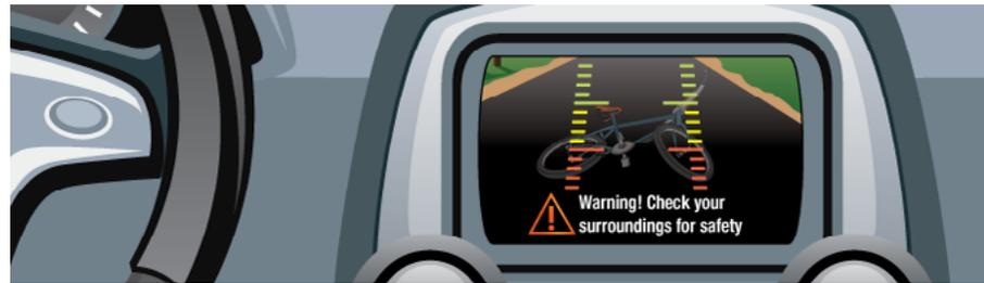
**How It Works:** When the driver shifts into reverse, the rear camera activates to show the area behind the vehicle. Depending on the vehicle, the display screen may be found on the center console, in the rearview mirror, in the sun visor, or in other locations.
