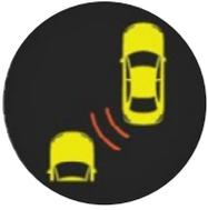
**Description:** Warns the driver of other vehicles driving in their blind spots through display of a symbol, sound, or vibration. They may provide an additional warning if a driver uses their turn signal when there are other vehicles in another lane.
