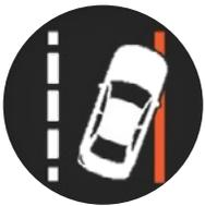
**Description:** Alerts a driver when they are drifting out of their lane using visual, vibration, or sound warnings. This feature can help alert a driver to steer back to the center of their lane if they mistakenly drift, helping to prevent a crash.
