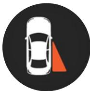
**Description:** Shows the driver an expanded view of a lane beside the vehicle when they use the turn signal or when they activate the feature manually. This feature shares similar uses to blind spot monitors.
