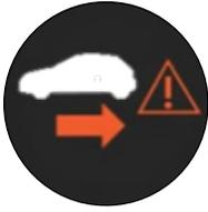
**Description:** Can apply the brakes if an obstacle is detected while reversing the vehicle. Helps the driver avoid a possible crash when the vehicle is moving in reverse.
