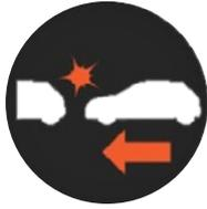
**Description:** Alerts drivers of an impending collision with a slower moving or stationary vehicle or object to the front so a driver can brake or swerve in time. The warning alone will not automatically brake for the driver. Forward collision warning scans the road ahead while driving.
