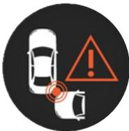
**Description:** Warns the driver if one or more vehicles are about to enter the backing path. Can detect vehicles that might be crossing during backing.
